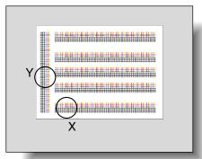
8 If the lines are shifted as shown at the right, touch to specify the desired negative adjustment for "X" (between -1 dot and -6 dots).
